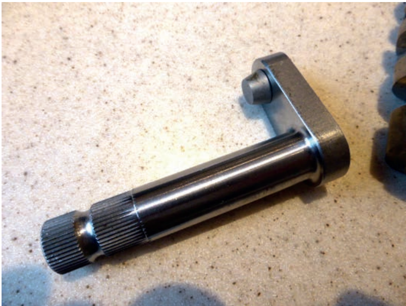
Photo 4: Steering shaft and worm in good condition
