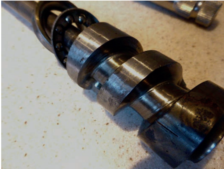
Photo 4: Steering shaft and worm in good condition
