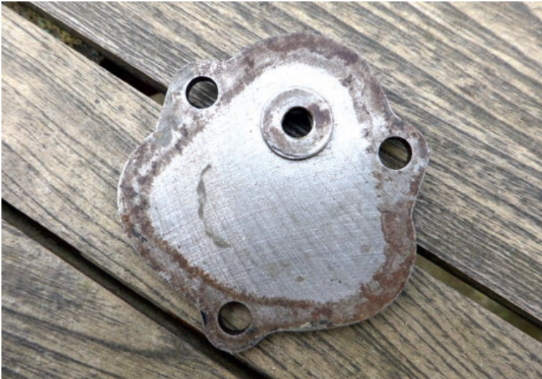
Picture 7: Cover plate with threaded bush for adjuster screw
