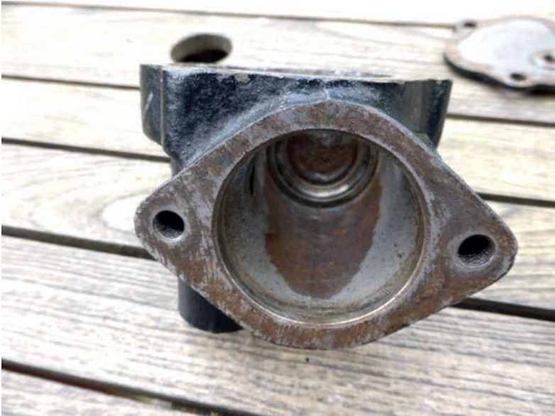
Photo 2: Bottom bearing race was OK
